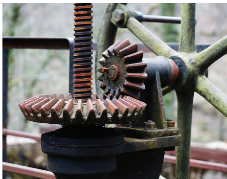
Bevel gear lifts a floodgate by means of a central screw.
