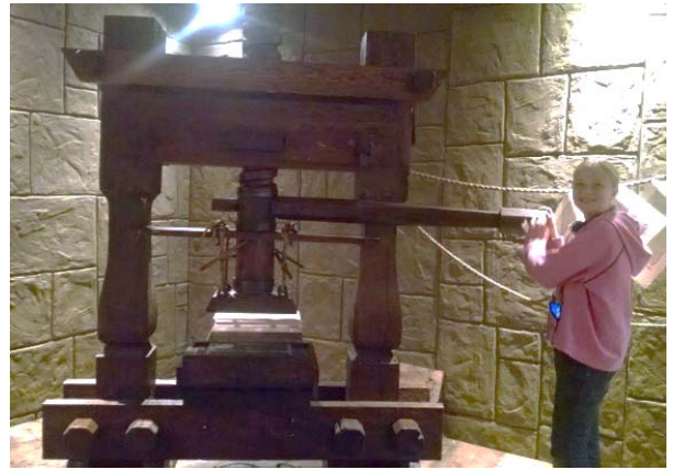
The girl is holding the handle of the press. When making a copy, the person operating the press walked around to spin the central section and lower the paper onto plates with the movable type.
