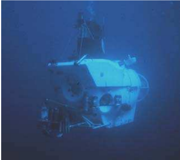
This submersible, called "Alvin," carries three scientists and has been to depths of more than 6,700 feet.
