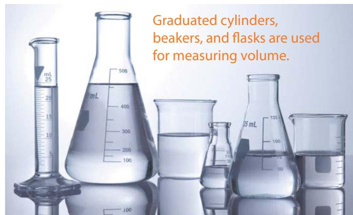
Graduated cylinders, beakers, and flasks are used for measuring volume.
