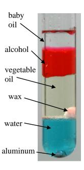
6. You see a glass tube with solids and liquids in it, as shown on the left. Order all the substances in the glass according to their densities. Start with the substance that has the lowest density and finish with the substance that has the highest density.
